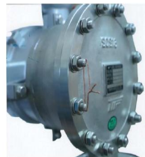
Wire seal arrangement for Back Cover
